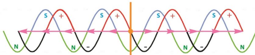
EM waves are a Quadrature waveform of Electric and Magnetic oscillations
